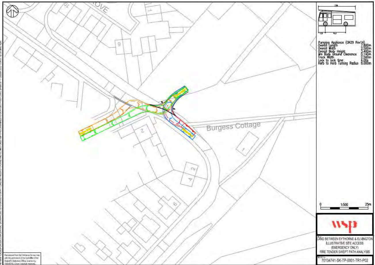
Figure 4-5 - Terrace Road- Illustrative Site Access Arrangement (Emergency Only) Swept Path Analysis
