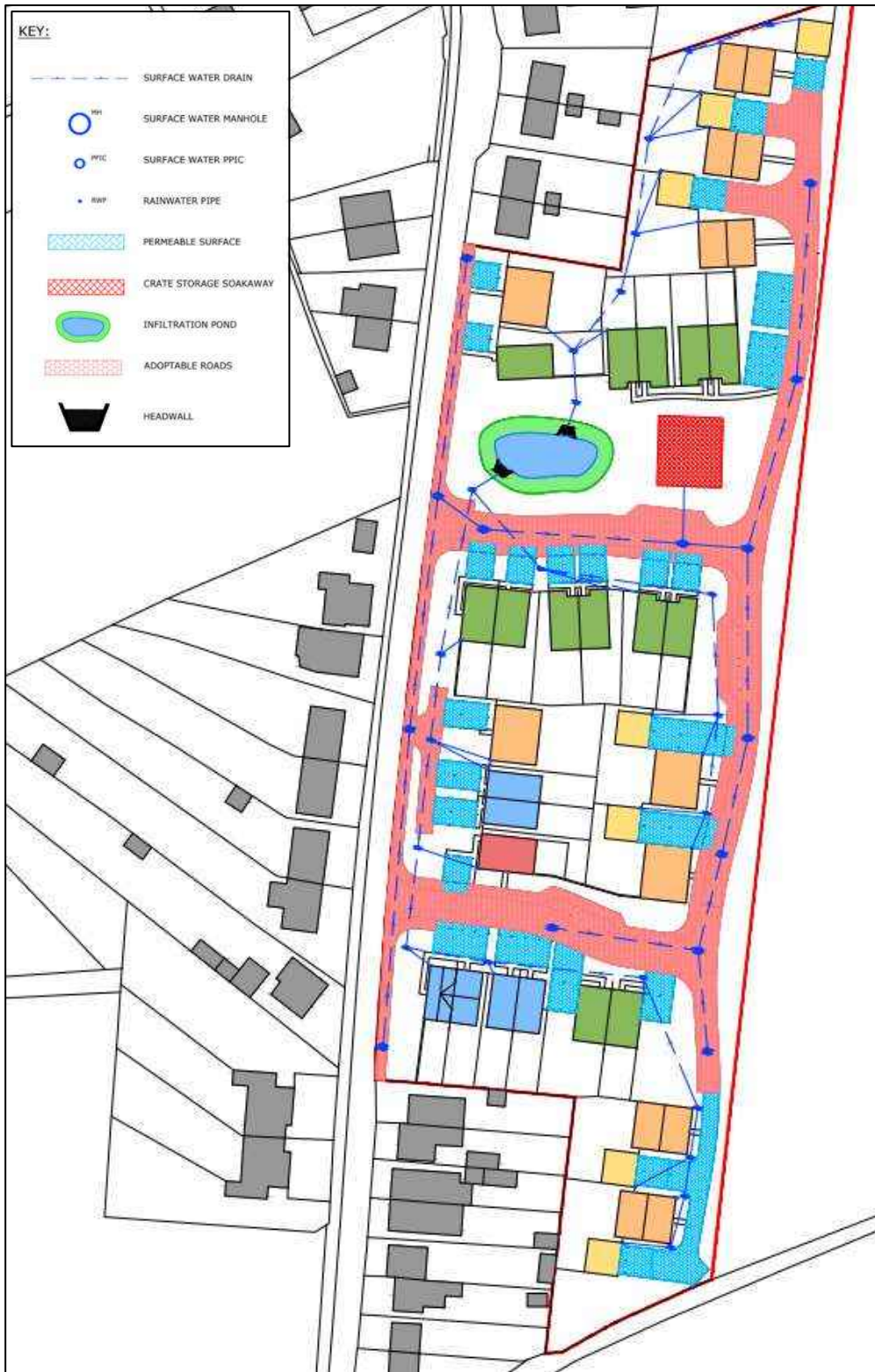
Figure 9.1 - Indicative drainage layout plan showing the proposed location of SuDS.
