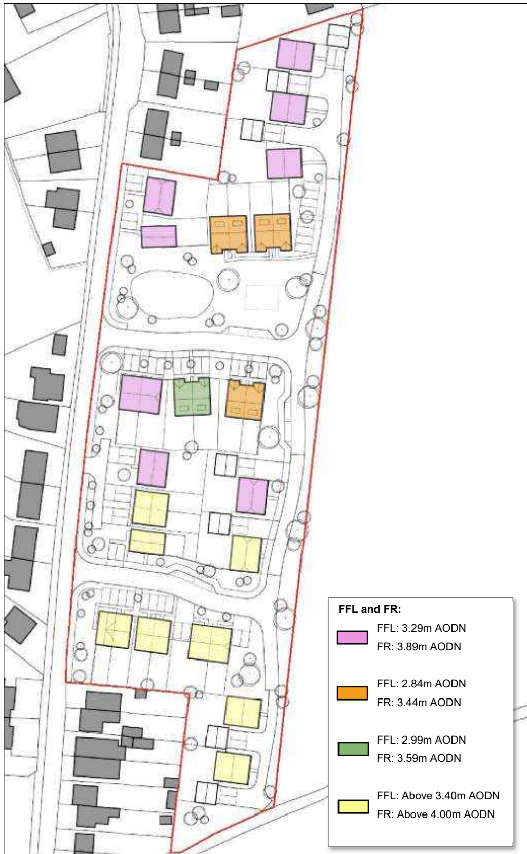
Figure 7.1 – Finished Floor Levels (FFLs) and the level Flood Resistance (FR) is effective to.
