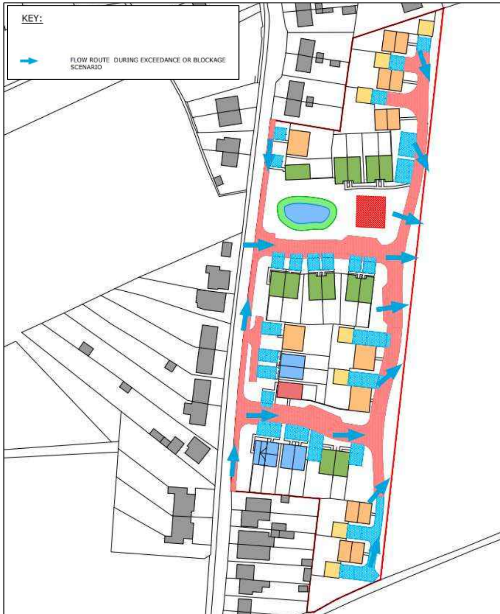
Figure 9.2 – Anticipated flow routes during an exceedance or blockage event (indicated by blue arrows)
