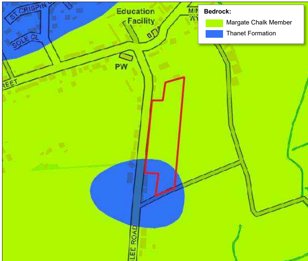
Figure 3.1 - Geology map showing the bedrock on the site (© British Geological Survey, mapping contains Ordnance Survey Data © Crown copyright and database right 2023).
