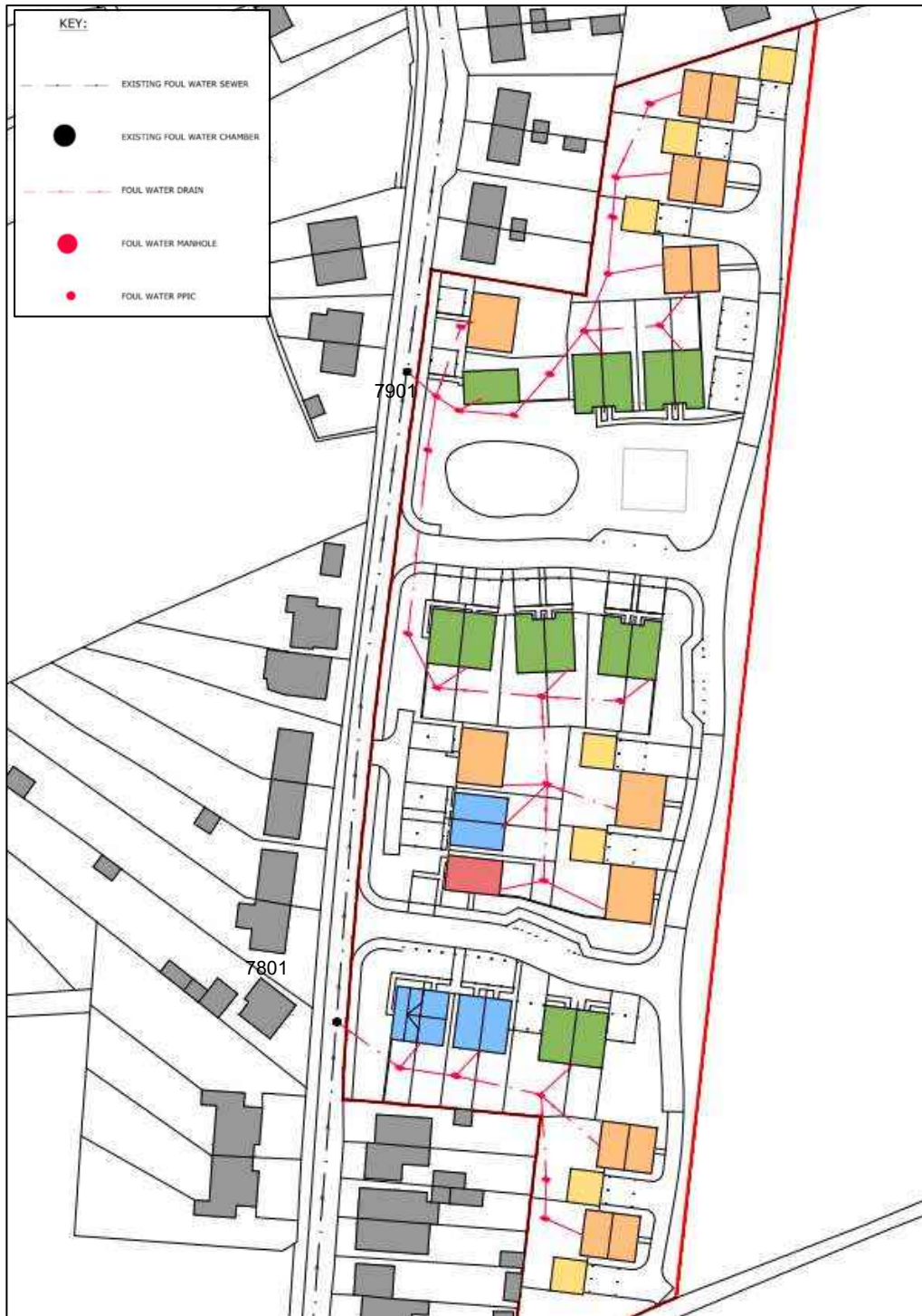
Figure 10.1 - Proposed connection to the foul sewer network.
