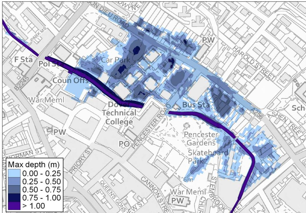
Figure 16 – Mitigation measure 1 maximum depth of flooding, 1:100 year event.
