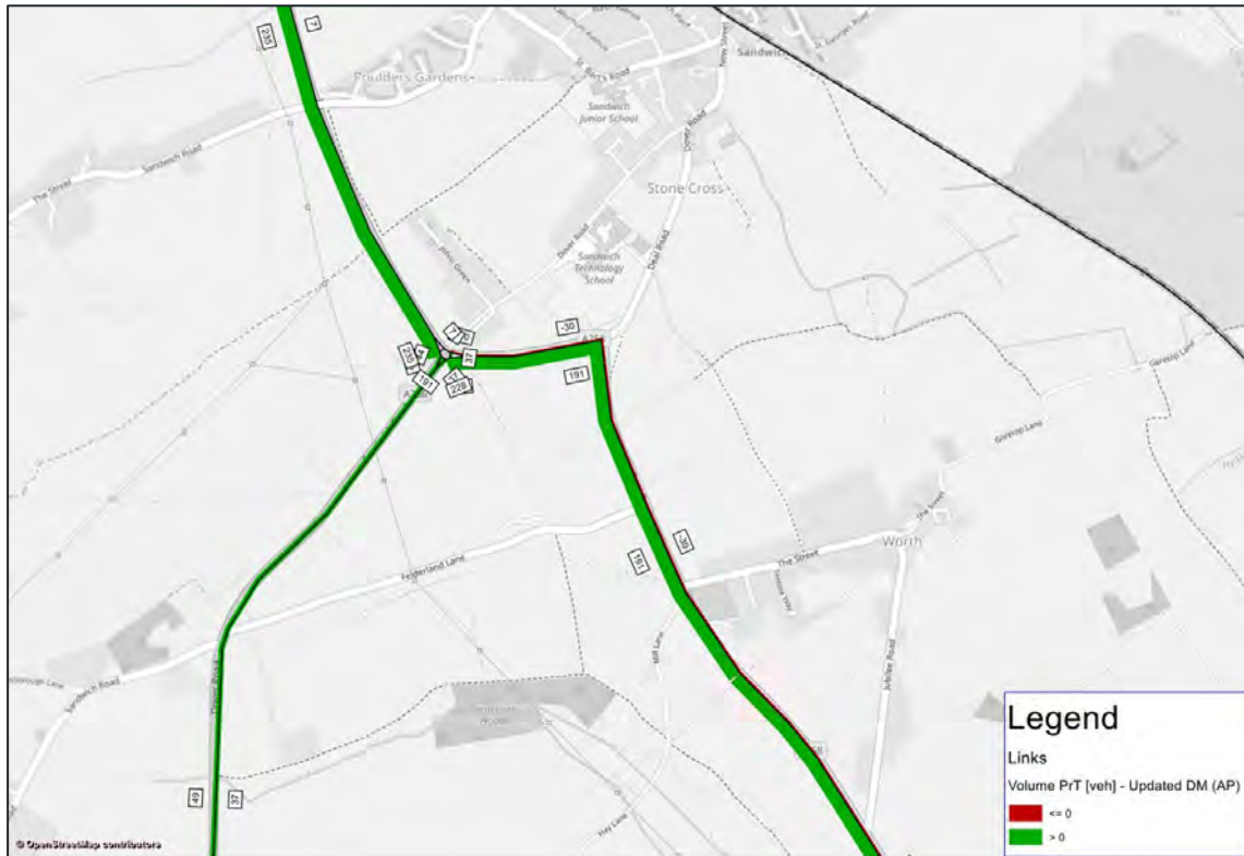
Figure 6-106: DDTM 2040 Refined Do Something - 2040 Do Minimum Flow Difference, A256/ Deal Road, PM Peak
