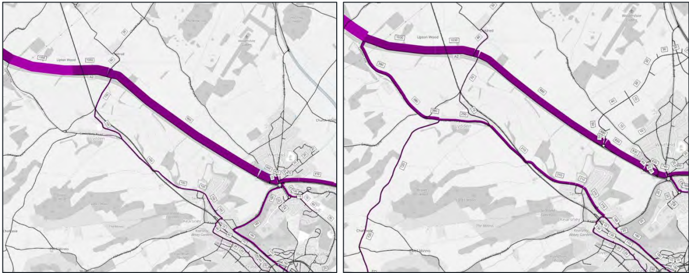
Figure 6-34: AM Peak Do Minimum vs Do Something, A2 Southbound Flow Bundle Comparison
