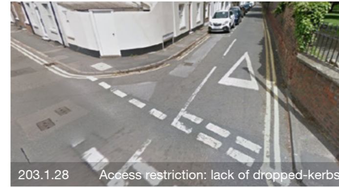
203.1.23 † Access restriction: lack of dropped-kerbs
