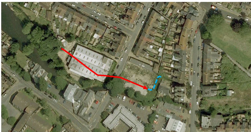
Figure 5 – Route of the culvert in the original EA model (red) and the double 90° bends. Image from GoogleEarth dated 2006.
